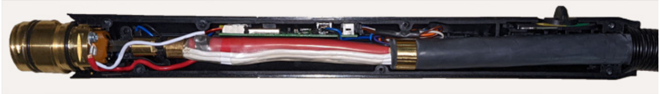
Figure 12 – Full-length machine torch components in correct positions
