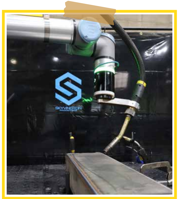
Skyvington makes long linear welds with the ESAB Cobot.
