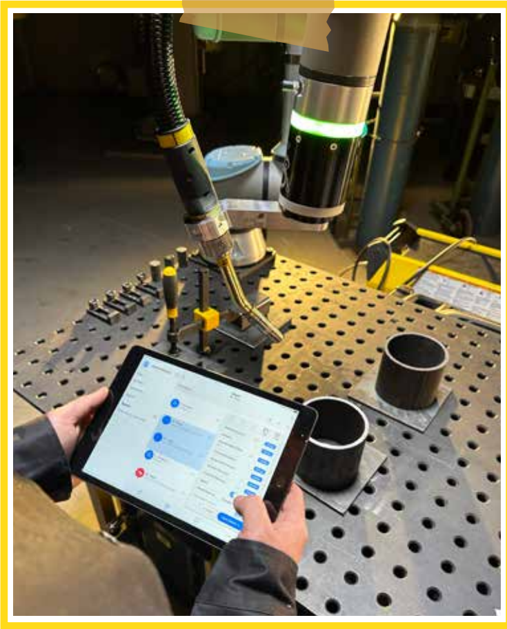
Users program the ESAB Cobot with a software app and standard tablet.
