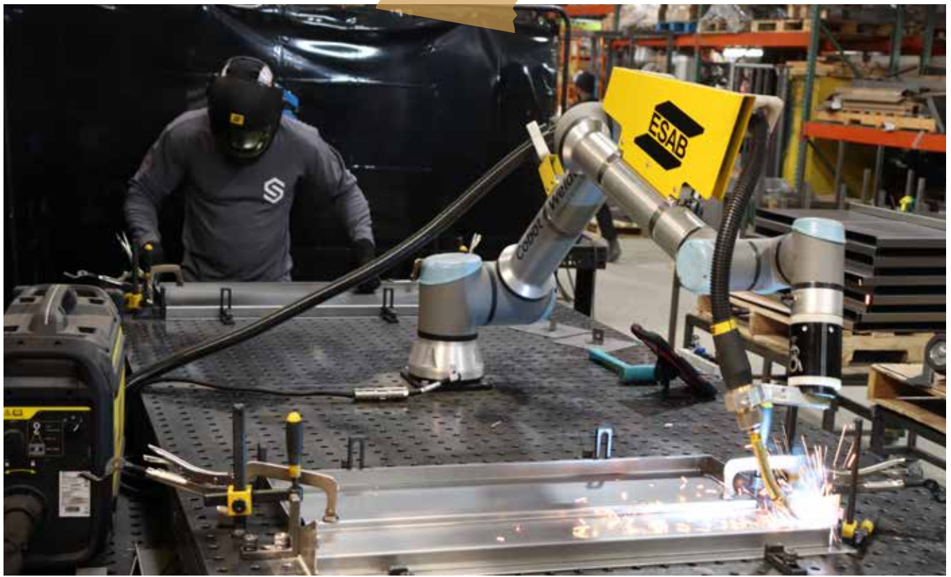
Skyvington Manufacturing set up the ESAB Cobot with a large Siegmund table so that it can weld on one side while an operator loads parts on the other.
